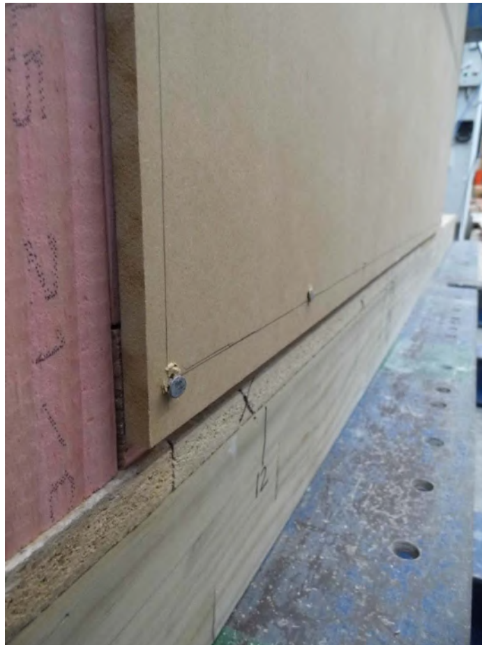
Figure 4. Typical Nail Movement as Observed Following Testing of 1200 mm MDF Sheathed Wall Panels
