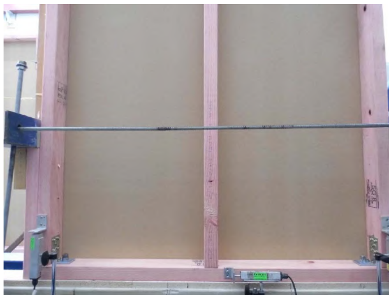
Figure 3. Daiken Customwood 1200 mm Long Specimen Showing GIB® HandiBrac® Hold-Downs
