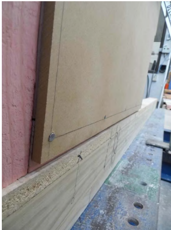
Figure 4. Typical Nail Movement as Observed Following Testing
